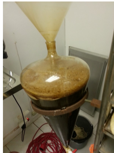
Illustration 14: The toluene emulsion before settling
