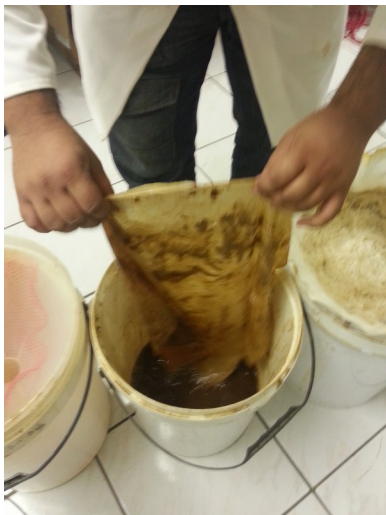
Illustration 56: Take the paper from the spent VTA for reuse
