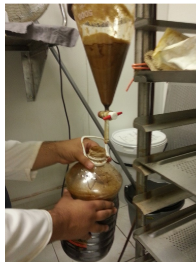
Illustration 19: Stopcock closed to keep the toluene emulsion in
