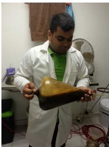
Illustration 16: Shake the funnel thoroughly
