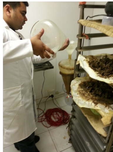
Illustration 30: Add the dilute HCl to the toluene emulsion
