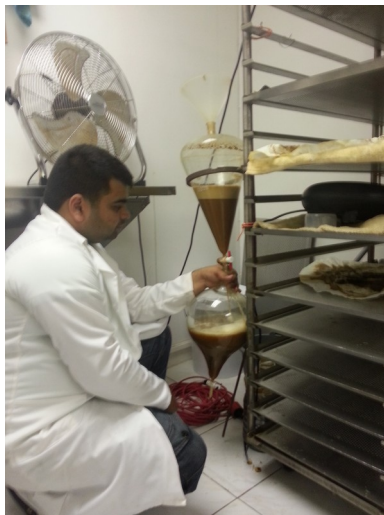
Illustration 34: Dispense the acid layer
