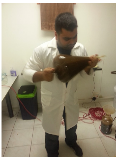
Illustration 21: Shake the funnel thoroughly
