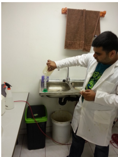
Illustration 28: Measure 30 mL of HCl
