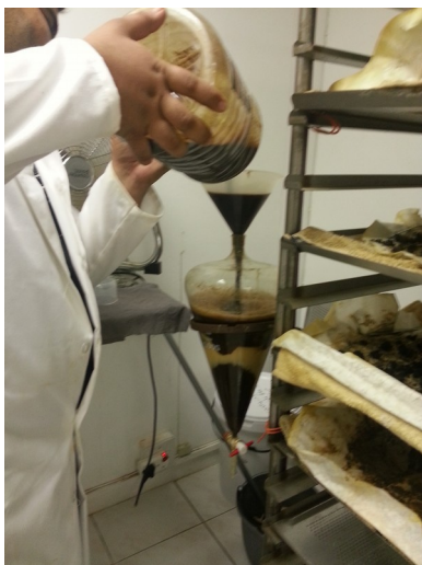
Illustration 45: Return VTA extract to separatory funnel
