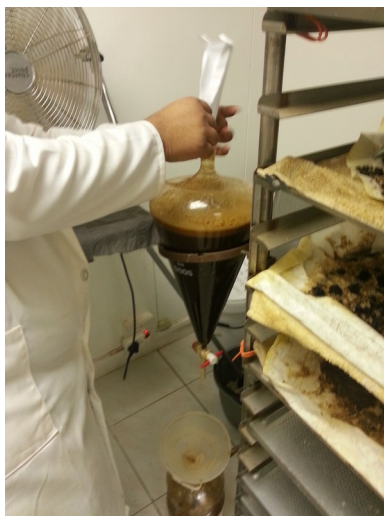
Illustration 46: Add 400 mg sodium acetate
