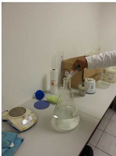
Illustration 29: Add the HCl to three liters of water
