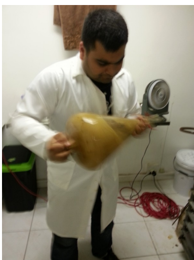
Illustration 31: Shake the funnel thoroughly
