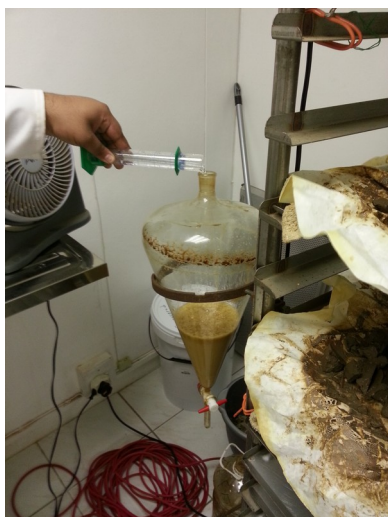
Illustration 9: Topping up the toluene emulsion
