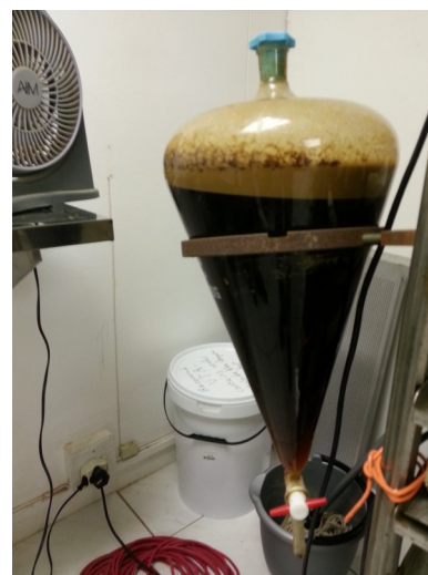
Illustration 22: The emulsion settled from the water wash
