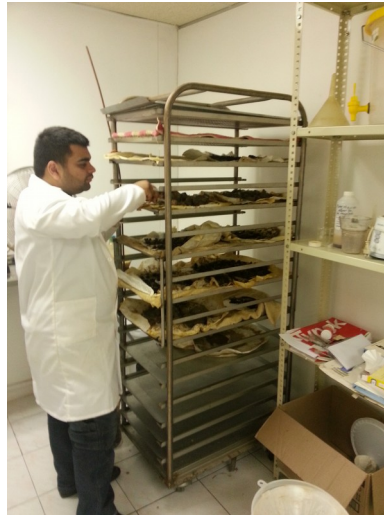
Illustration 52: Dry the recovered VTA
