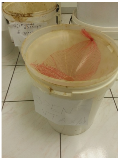
Illustration 57: Funnel lined with a plastic net
