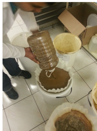
Illustration 50: Filter the recovered VTA
