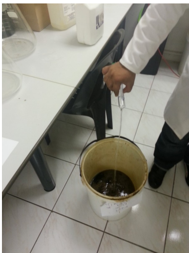
Illustration 61: Add ammonia to the HCl extract of VTA
