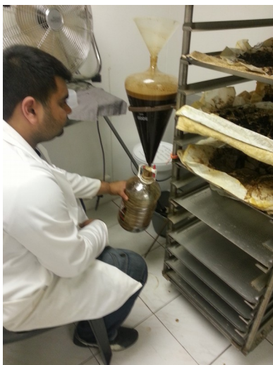
Illustration 17: Settled toluene emulsion before separation
