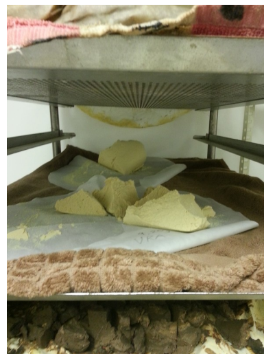
Illustration 49: Dry the VRA in a stream of air
