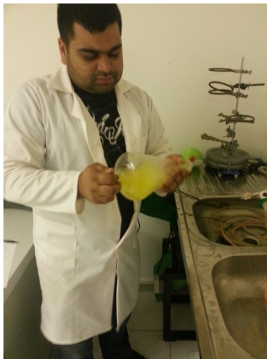
Illustration 89: Shake the stoppered separatory funnel thoroughly
