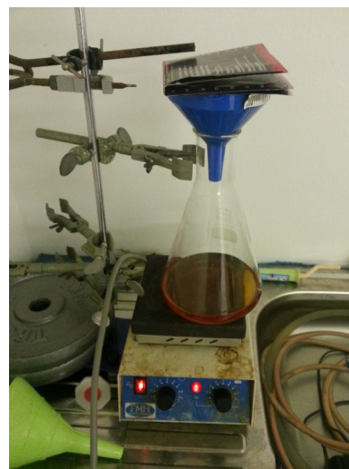
Illustration 108: Keep the methanol in the filter hot by covering it, and heat the flask but don't let it boil away
