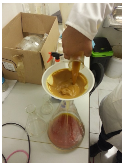
Illustration 29: Filter the PVTA HCl from the acetone solution of VRA
