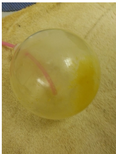
Illustration 124: Dry the crystals with a stream of air from an aquarium pump
