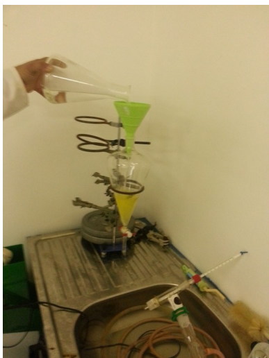
Illustration 88: Add the dilute HCl to the naphtha mother liquor
