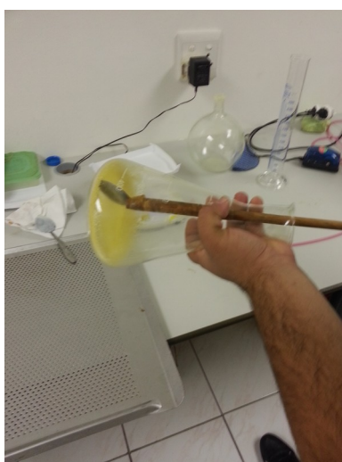
Illustration 113: Gently scrape the voacangine crystals from the flask with a scoop or spoon
