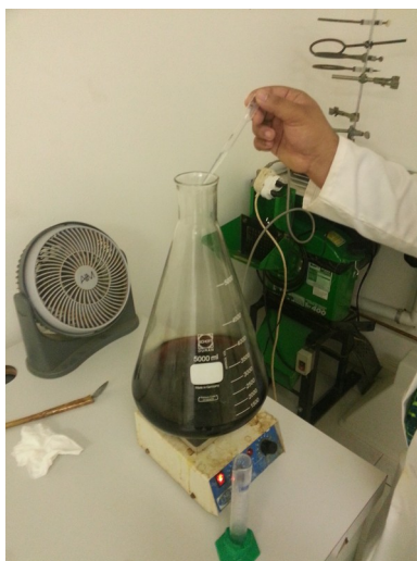
Illustration 18: Add HCl dropwise to let precipitation start gradually
