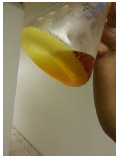
Illustration 111: Crystals of voacangine after refrigeration
