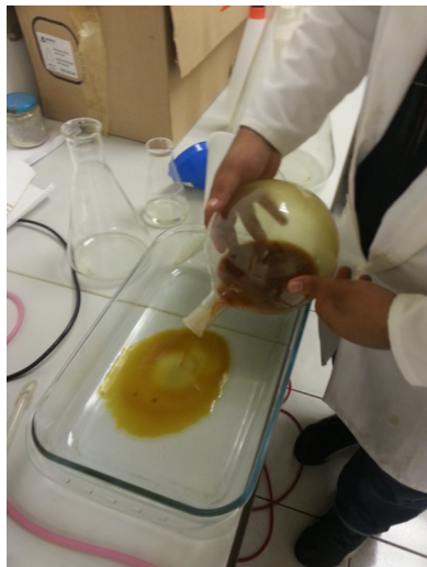
Illustration 38: Pour the contents of the distilling flask into a casserole dish
