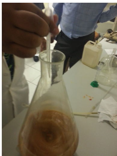
Illustration 20: Add HCl in 1 mL portions
