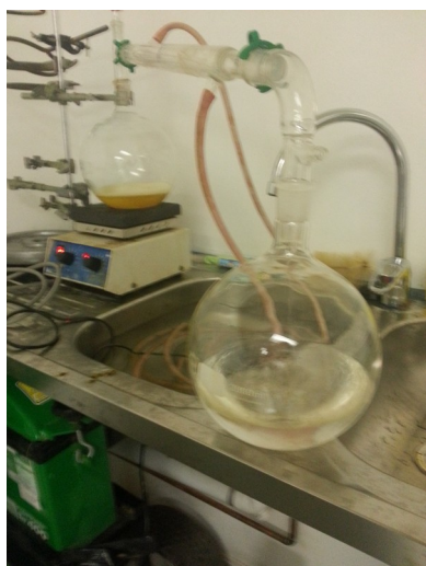
Illustration 67: Distill most of the naphtha
