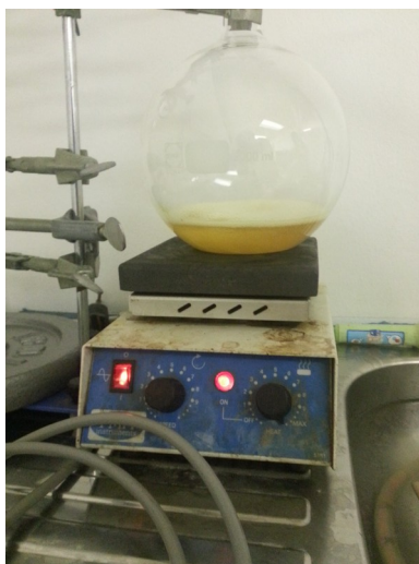
Illustration 68: Stop distilling when about 200 mL of VRA extract remains.
