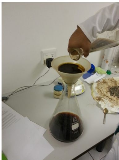
Illustration 11: Rinse the filter with acetone
