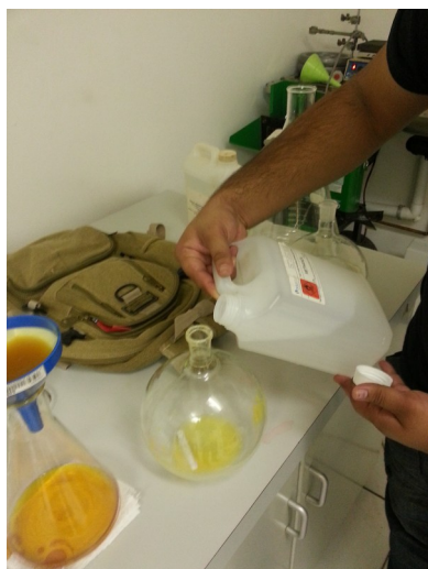
Illustration 106: Add ~50 portions of methanol and heat the flask to dissolve the remaining voacangine
