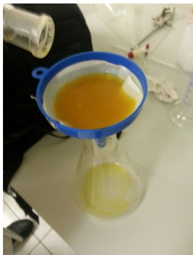
Illustration 103: Filter the fine solid impurity out of the hot solution
