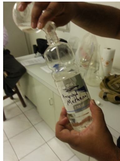
Illustration 117: Put the distilled methanol in the original container to save it for reuse
