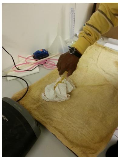
Illustration 121: Decant the mother liquor from the second crop onto a wad of paper towels
