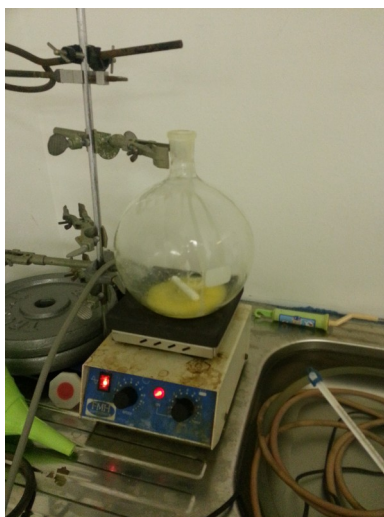
Illustration 107: Heat each portion of methanol to simmering but don't let it boil away
