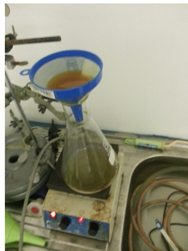
Illustration 105: Keep the filtrate hot but don't let it boil away
