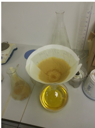
Illustration 62: Wait until the naphtha finishes draining from the filter
