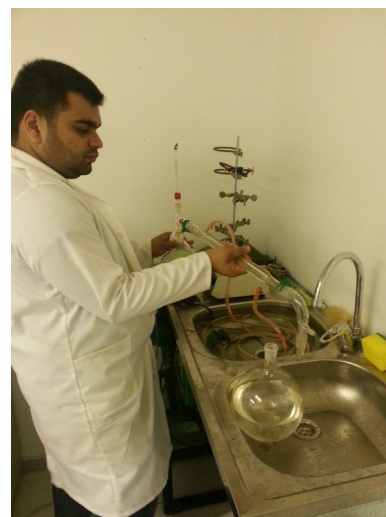
Illustration 37: Carefully remove the receiving flask and the boiling flask from the condenser
