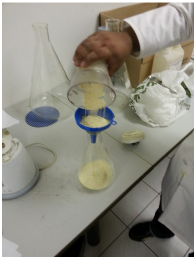
Illustration 56: Add the VRA/diatomaceous earth to an Erlenmeyer flask
