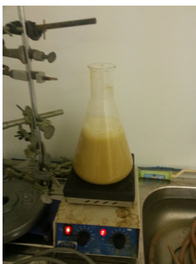
Illustration 60: Heat the mixture to boiling but do not let much liquid boil away
