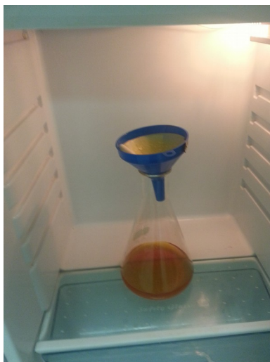
Illustration 110: Refrigerate the flask to increase the yield of crystals
