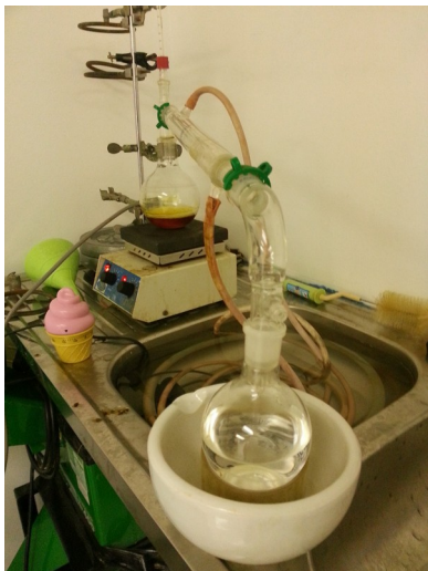
Illustration 115: Distill about 75% of the original volume – this picture is less than full scale.
