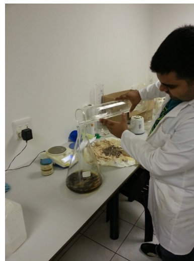
Illustration 3: Add one liter of acetone to the flask
