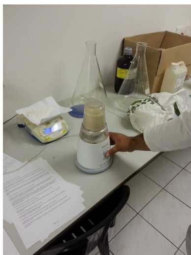
Illustration 53: Grind the equal amounts of VRA and diatomaceous earth until all the VRA is a fine powder
