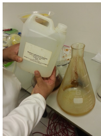
Illustration 31: Add about 100 mL of acetone to the flask to rinse it
