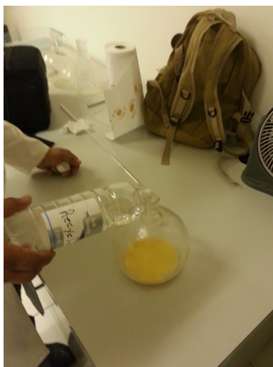
Illustration 83: Rinse the crystals of voacangine with a bit of clean naphtha
