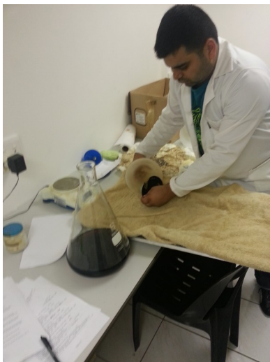
Illustration 14: Remove the drained filter paper
