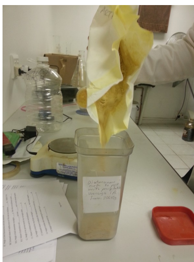
Illustration 77: Store the used diatomaceous earth until it can be added to precipitated VTA
