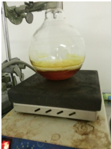
Illustration 116: At the end of the distillation there should not yet be solid in the concentrated mother liquor
