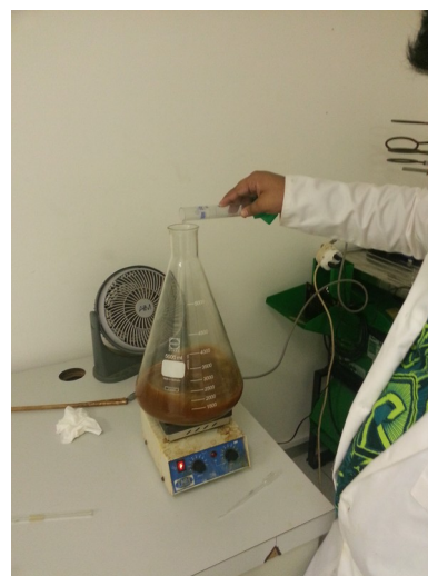
Illustration 19: Once the precipitation starts, the rest of the HCl can be added more quickly
