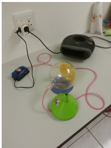
Illustration 85: Dry the voacangine with a stream of air from an aquarium pump and gentle warming from a heater
