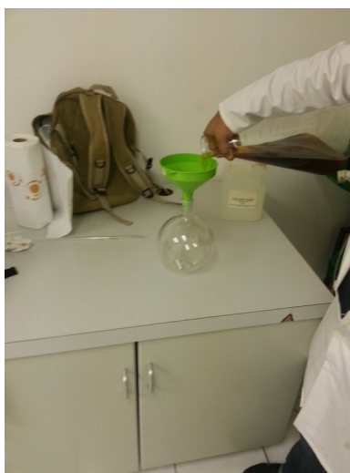
Illustration 30: Pour the filtrate into a distilling flask or, better, filter into it directly
