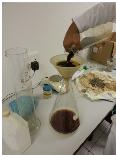
Illustration 8: Filter the impurity from the solution
