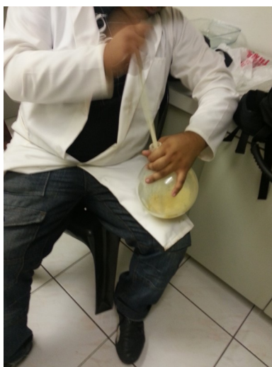
Illustration 86: Use a rod to gently break up the mass of crystals and scrape them from the glass to facilitate drying or to remove them from the flask
