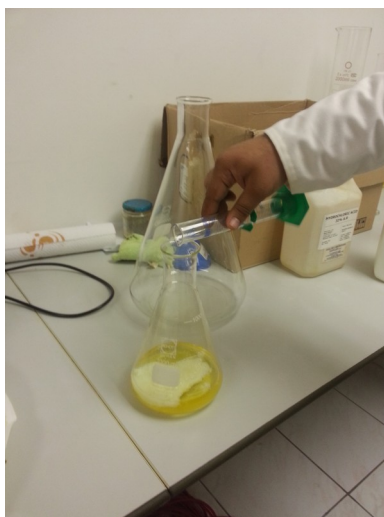
Illustration 92: Add ammonia to the yellow aqueous layer to make it basic
