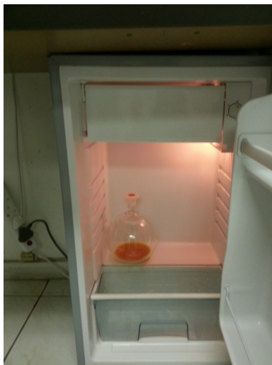
Illustration 80: Place the flask in a refrigerator for at least six hours
