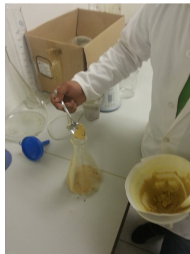
Illustration 63: Return the diatomaceous earth that gets into the filter to the flask
