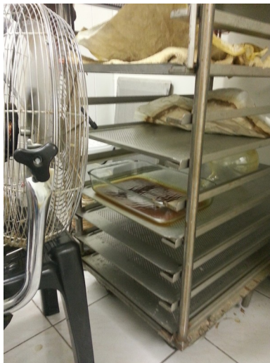
Illustration 39: Put the casserole dish in a breeze so the acetone evaporates
