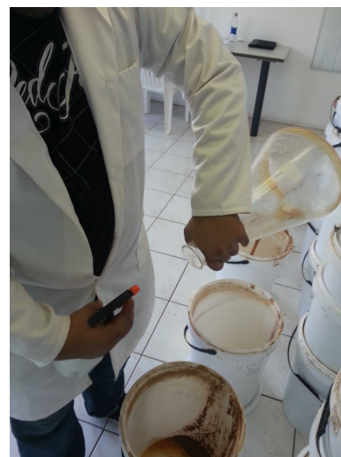
Illustration 34: Rinse the PVTA HCl adhering to the flask into bark extract with water
