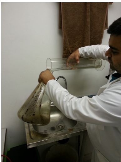
Illustration 10: Use the acetone to rinse the flask
