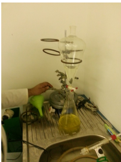
Illustration 91: Remove the stopper and drain the lower yellow layer
