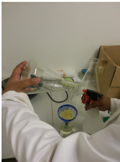
Illustration 95: Rinse any remaining solid into the filter with a spray of water
