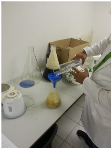
Illustration 57: Add petroleum naphtha to the flask
