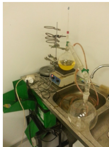
Illustration 66: An empty round flask to receive the distilled naphtha
