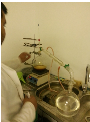
Illustration 36: Stop the distillation when approximately 300 mL remain
