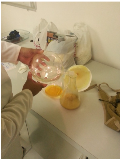
Illustration 70: Extract the diatomaceous earth again with the distilled naphtha
