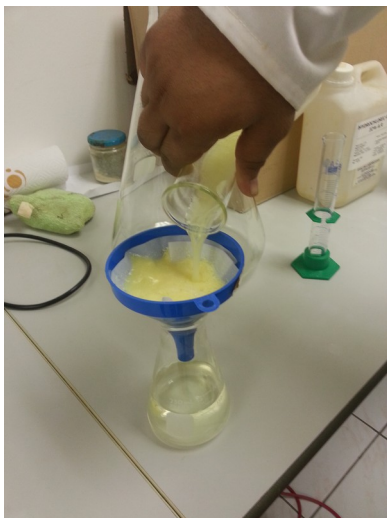
Illustration 94: Filter the recovered voacangine through a weighed paper
