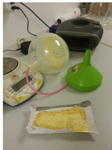
Illustration 87: If the voacangine is removed from the flask, let it dry completely before recording its weight
