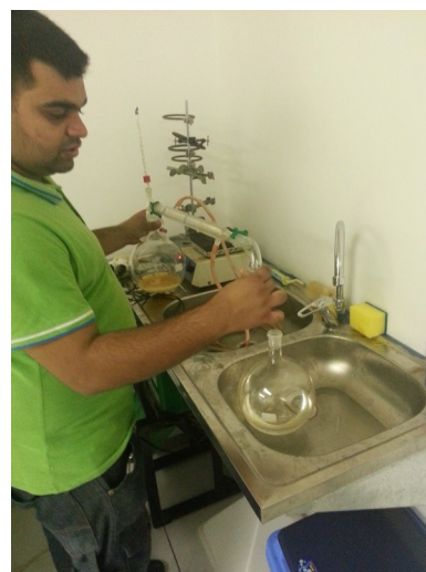
Illustration 69: Carefully dismantle the still
