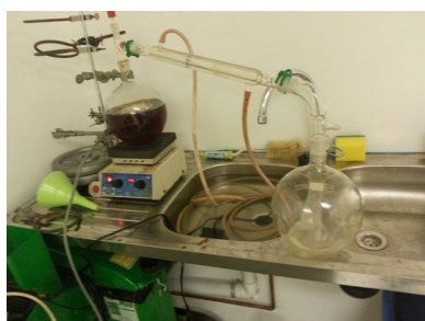
Illustration 35: Distill the acetone from the VRA solution
