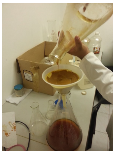
Illustration 32: Rinse the PVTA HCl with acetone
