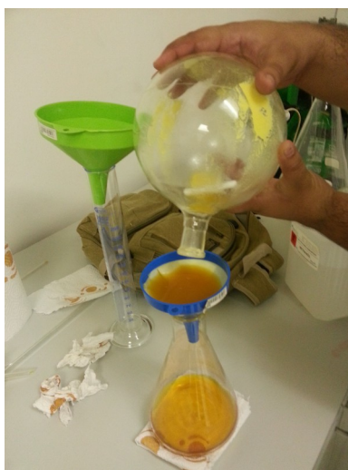
Illustration 104: Keep undissolved voacangine in the round flask for the next step
