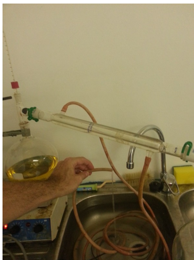
Illustration 65: A condenser to recover the naphtha as it boils away
