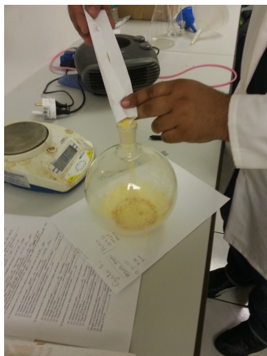
Illustration 98: Put a carefully weighed quantity of voacangine in a flat-bottom round flask
