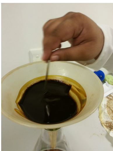
Illustration 12: Stir the solid so it is all exposed to the acetone
