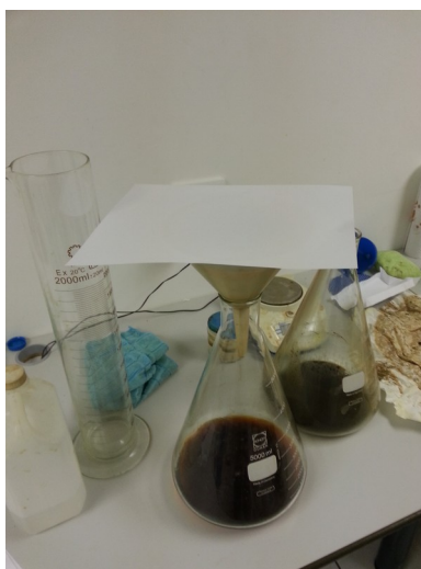
Illustration 9: Cover the funnel to prevent the acetone from evaporating
