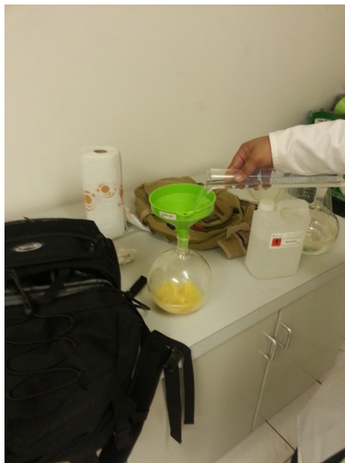
Illustration 99: Add the measured amount of methanol to the flask
