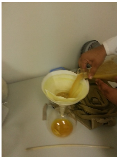
Illustration 71: After boiling, filter through the same paper used for the diatomaceous earth previously
