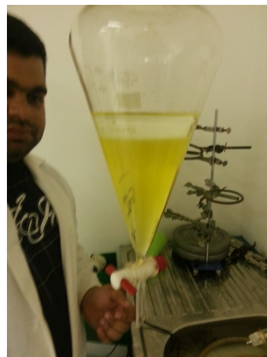
Illustration 90: Wait for the layers to separate
