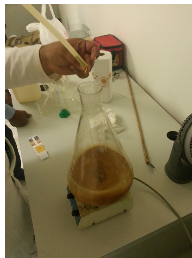
Illustration 22: Apply the sample to pH test paper
