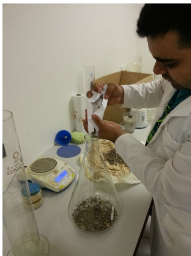
Illustration 2: Pour the PVTA into an Erlenmeyer flask
