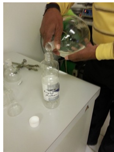
Illustration 59: Save the distilled methanol for reuse in the next recrystallization.
