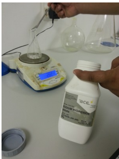
Illustration 29: Weigh 60 grams of sodium hydroxide into the flask.
