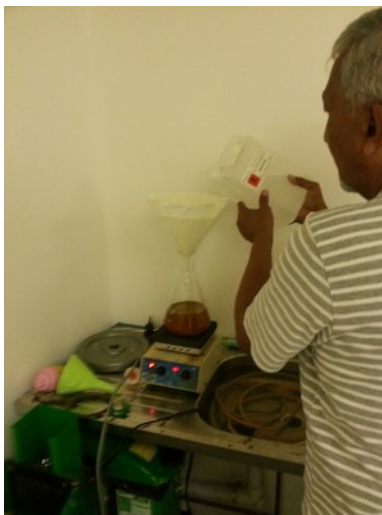
Illustration 49: Add portions of methanol as needed to dissolve most of the solid.
