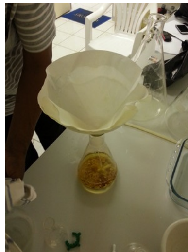
Illustration 47: Let all the rinse drain into the flask.
