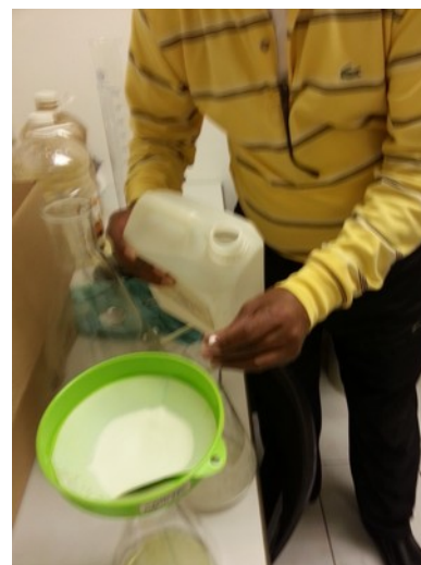
Illustration 72: Rinse the stir bar and flask with acetone, and use this to rinse the product in the filter.
