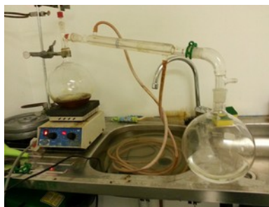
Illustration 58: Continue the distillation until the volume remaining is about 25% of the original.
