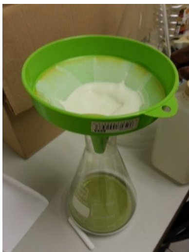
Illustration 73: Let all the acetone drain from the filter.
