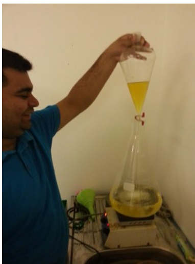
Illustration 23: Add the solution from the separatory funnel to the boiling acid slowly enough that it does not overflow.
