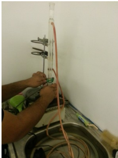
Illustration 7: Attach a reflux condenser to the flask.
