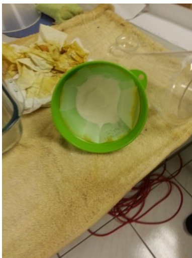
Illustration 74: Set the funnel on its side to let the acetone evaporate slowly.
