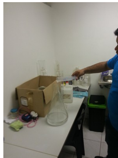
Illustration 21: Add the hydrochloric acid to the water in the flask.
