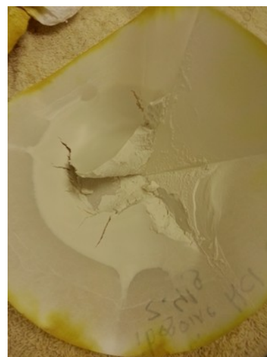
Illustration 75: Move the paper onto the towel to allow the last of the acetone to evaporate.
