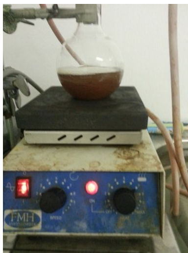
Illustration 11: Continue boiling the mixture on a heat setting of 7 (your setting may vary).
