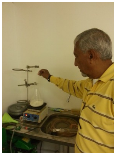
Illustration 65: During the addition of acid the solution will become very cloudy.
