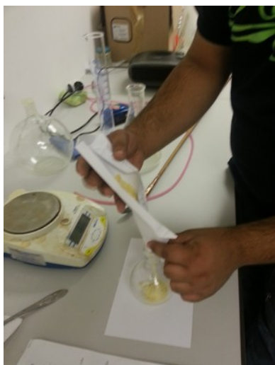
Illustration 1: Pour the weighed voacangine into the flask
