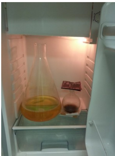
Illustration 28: Refrigerate the yellow solution for six hours.
