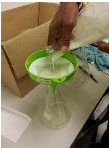
Illustration 71: Filter the ibogaine HCl product from the acetone.
