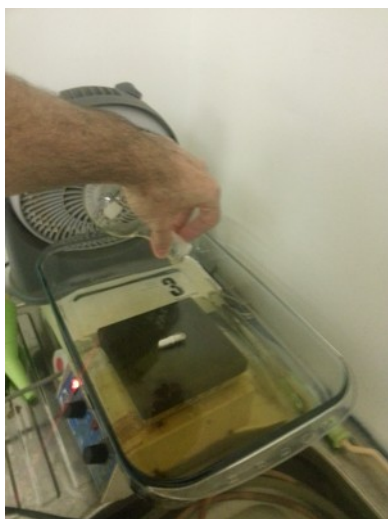
Illustration 13: Pour the hot solution and stir bar into a glass casserole dish in front of a fan.
