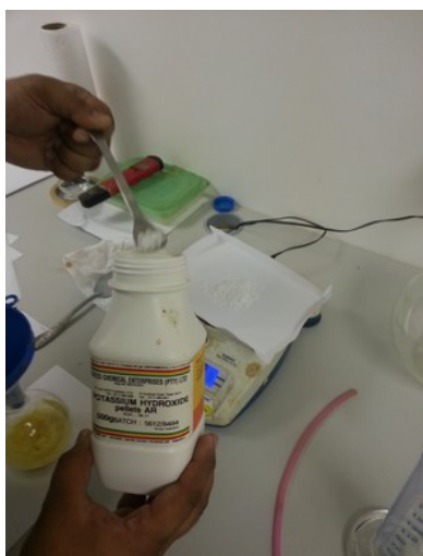
Illustration 4: Weigh out the potassium hydroxide.
