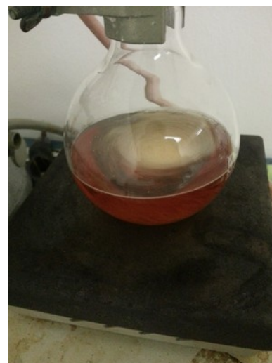
Illustration 12: After about an hour the solid should dissolve to give a clear tea-colored solution.
