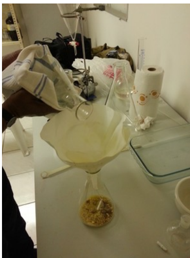
Illustration 46: Rinse the filter paper with methanol.
