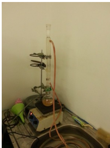
Illustration 8: Seal the flask to the condenser with teflon tape and a Keck clamp,
