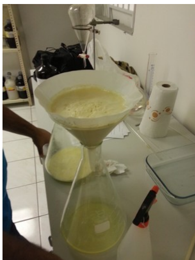
Illustration 36: Filter the ibogaine from the yellow solution.
