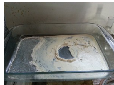
Illustration 15: All the liquid should evaporate to leave a tan or light-yellow paste.
