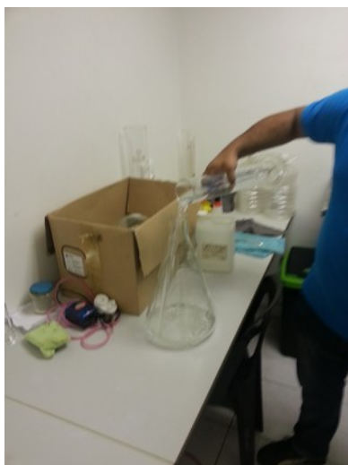
Illustration 19: Measure four liters of water and add it to a five liter Erlenmeyer flask containing a stir bar.
