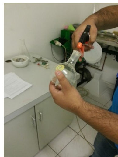
Illustration 18: Rinse the residue from the reaction flask into the casserole dish.
