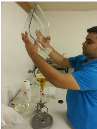
Illustration 22: Add the solution from the casserole dish to the separatory funnel.
