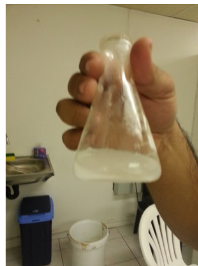
Illustration 31: Swirl the flask until the sodium hydroxide has dissolved.
