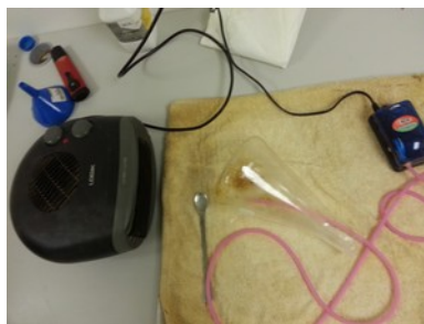
Illustration 55: Warm the flask while using a stream of air from an aquarium pump to dry the ibogaine crystals.
