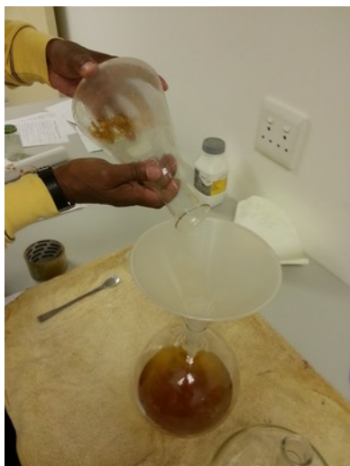
Illustration 54: Decant the liquid to leave the crystals behind.
