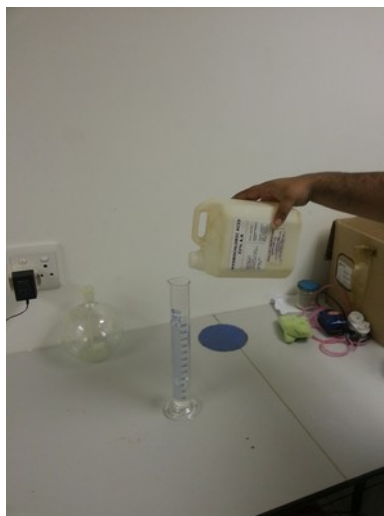
Illustration 20: Measure out 240 mL of concentrated hydrochloric acid
