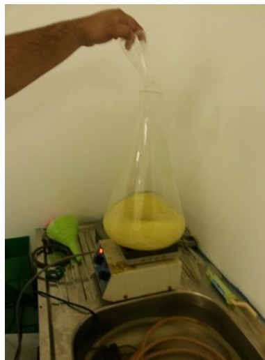
Illustration 33: A fluffy precipitate of ibogaine base appears as the sodium hydroxide is added.
