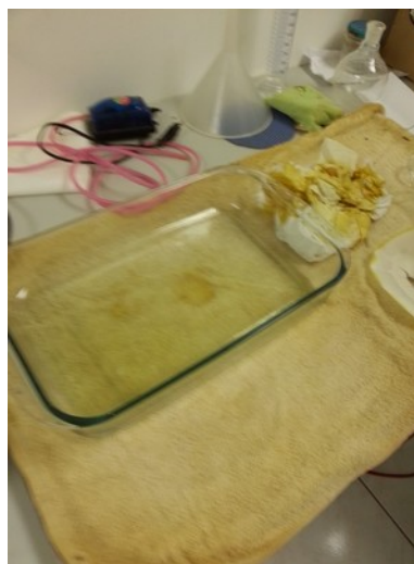
Illustration 77: Let the acetone solution evaporate in a well ventilated area.
