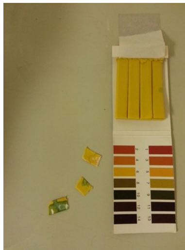
Illustration 68: Stop adding acid when the pH reaches 3. The pHs shown here are about 9, 7 and 6 from bottom to top.
