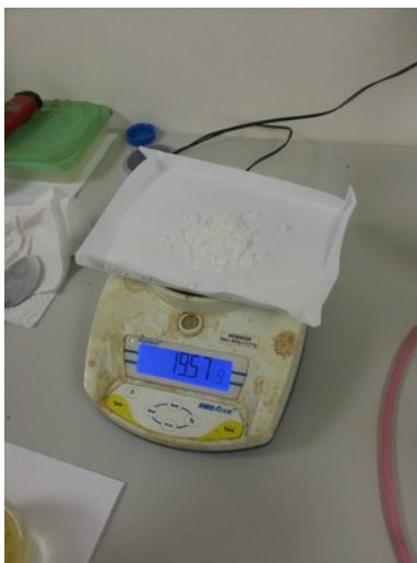
Illustration 5: When finished weighing, pour the potassium hydroxide into the flask.
