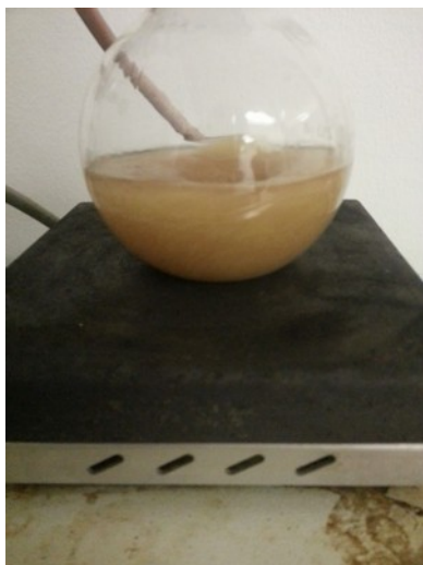
Illustration 10: Heat the stirring mixture to boiling.
